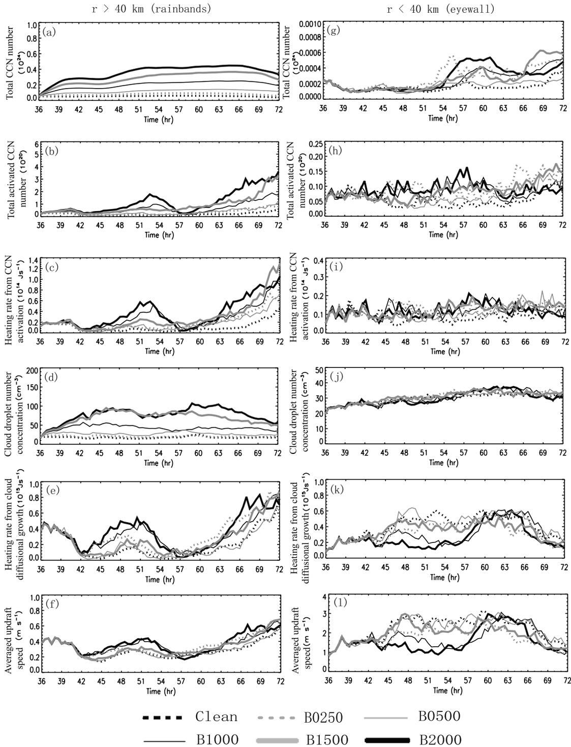
**Figure 3.** (a) and (g) Temporal evolution of total CCN number, (b) and (h) total activated CCN number, (c) and (i) heating rate from CCN activation, (d) and (j) cloud number concentration, (e) and (k) heating rate from cloud diffusional growth, and (f) and (l) averaged updraft speed for the (left) rainbands and (right) eyewall using the 40 km radius as a threshold.
